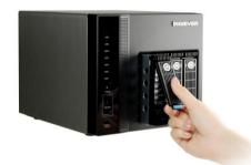
② Install the hard disk in each tray and lock the disk with four screws. Ensure the disk holes match the holes at the base of disk tray.
